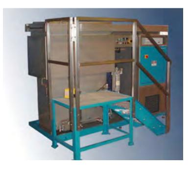
Greco Brothers Ultrasonic Vapor-Spray Degreasers are designed and built to provide years of efficient, reliable service when using chlorinated solvents, n-propyl bromide, or the new HFE and HFC solvent blends. All Greco Brothers solvent vapor degreasers meet recent EPA and NESHAP guidelines for currently accepted degreasing solvents.
