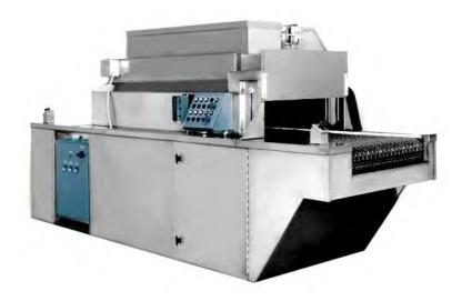
Greco Brothers Conveyorized Hot Air Drying Systems incorporate a stainless steel mesh conveyor that carries parts through a heated convection drying chamber. These systems are best suited for operations with high production requirements.
