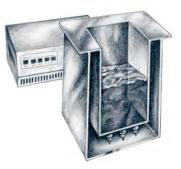
These systems are offered in the sizes ranging from 10" x 12" x 10" deep, to 24" x 48" x 20" deep. They include the transducerized tank, sweep frequency generator, thermostatically controlled heat, and connector cables. All systems are available in frequencies of 25 or 40 kHz. Stainless steel stands, covers, and filtration systems are optionally available.
