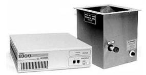
The standard batch tank is the simplest ultrasonic cleaning system available. It consists of an ultrasonic generator and a transducerized cleaning tank. The transducerized tank is constructed of stainless steel, with the transducer elements bonded to the tank bottom. The ultrasonic energy is directed upward through the tank.
